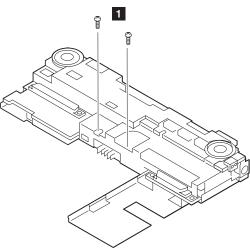
Turn the system board upside down. Then remove any metal tape holding the card.
